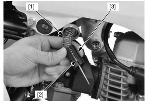
Be careful not to damage the jet needle when installing the throttle valve [1] into the carburetor body.
