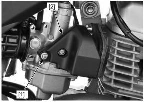
Disconnect the carburetor heater connector [1] and ground wire connector [2].
