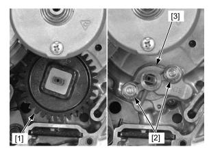
Remove the dowel pins [1] from the oil pump body.
