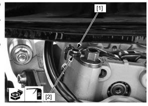
Install a new gasket [1] into the cylinder head cover groove.
