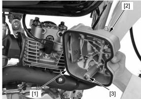
Remove the dowel pin [1] and O-ring [2] from the camshaft holder.
