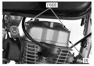
Remove the gasket [1] from the cylinder head cover [2].
