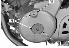
Rotate the crankshaft counterclockwise and align the "T" mark [1] on the flywheel with the index notch [2] on the left crankcase cover.
