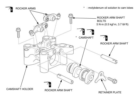
Apply engine oil to the rocker arm [1] inner surfaces, rollers and rocker arm shaft [2] entire surfaces.
