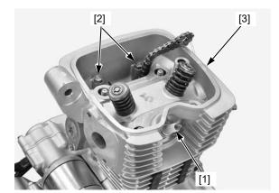
Remove the cylinder head gasket [1] and two dowel pins [2].
