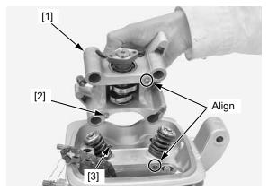
Apply engine oil to the threads and seating surfaces of the camshaft holder special nuts [1].
