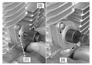
Remove the cam chain tensioner lifter [1] and gasket [2] from the cylinder.
