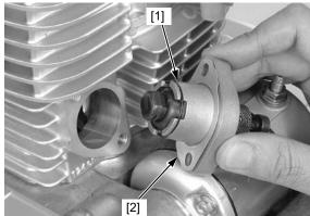
Check the cam chain tensioner lifter operation:
