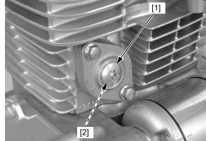
Turn the cam chain tensioner lifter shaft [1] clockwise fully and secure it using the special tool.
