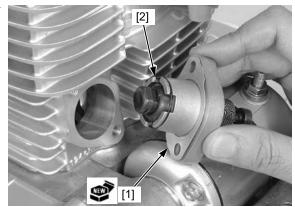
Install the two mounting bolts [1] and tighten them.
