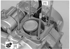
Apply engine oil to the cylinder wall, piston outer surface and piston rings.
