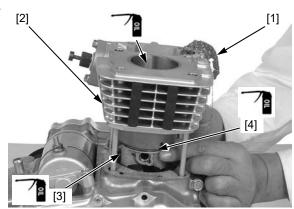
Insert the cam chain guide [1] into the cylinder and crankcase grooves [2].
