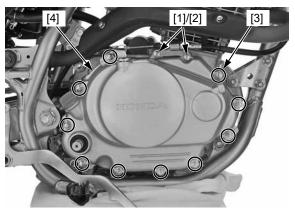
Remove the two dowel pins [1] and gasket [2].
