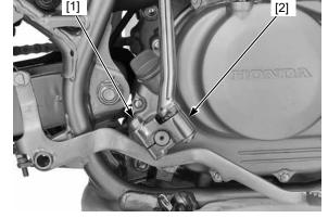
Remove the brake pedal return spring [1]. Disconnect the brake rod from the brake arm (page 15-4), then lower the brake pedal down.
