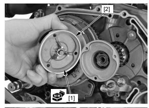
Install the oil filter rotor cover [1] and screws [2]. Tighten screws to the specified torque.
