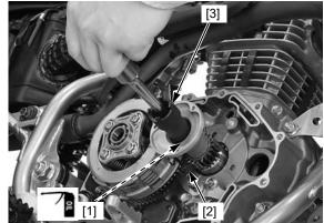
Install a new gasket [1] onto the oil filter rotor cover [2].
