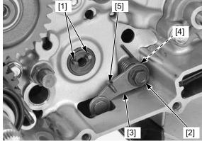
Inspect the gearshift spindle oil seal [1] for deterioration or damage, replace if necessary.
