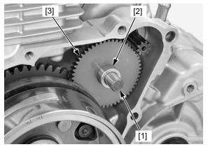
Hold the flywheel with the special tool and loosen the flywheel nut [1].
