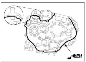
Install the two dowel pins [1]. Install the left crankcase over the right crankcase.
