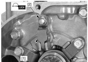
Install the cam chain [1] and cam chain guide [2]. Install the setting plate [3] with the two bolts [4] and tighten the bolts.
