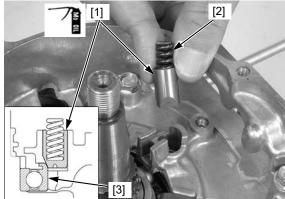
Apply locking agent to the push plug plate bolt threads. Install the push plug plate [1] and bolt [2], and then tighten the bolt to the specified torque.
