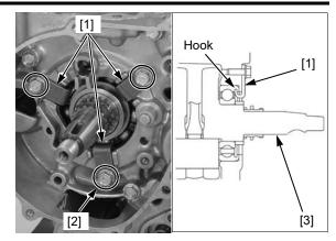
Apply molybdenum oil solution to the push plug entire surface.
