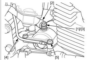
Remove the rubber caps [1] from the upper engine hanger plates.
