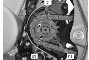
Install the gearshift pedal [1] on its original position as marked during removal.
