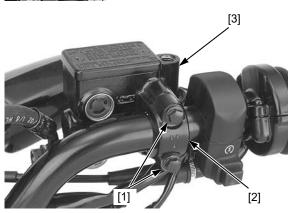
XL125LK: Remove the bolts [1], holder [2] and brake lever bracket [3].
