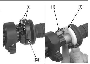
Remove the right handlebar switch housing screws [1]. Remove the right handlebar switch housing [2] from the handlebar.
