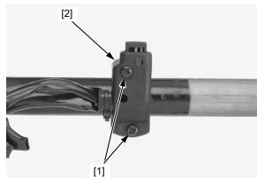
Disconnect the clutch switch connectors [1] from the clutch switch.
