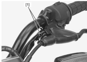
Remove the clutch lever holder screws [1], bracket [2] and holder [3].
