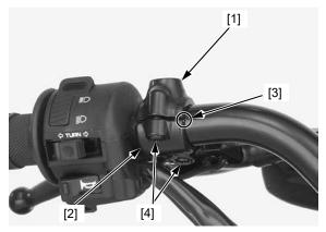
Connect the clutch switch connectors [1] to the clutch switch.
