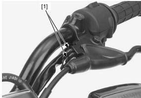
Install the right handlebar switch housing [1] by aligning its locating pin [2] with the hole [3] in the handlebar.
