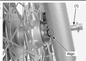
Install and tighten the front axle nut [1] to the specified torque.
