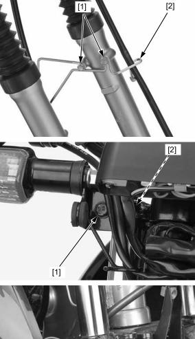
Loosen the top bridge pinch bolt [1].
