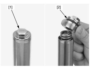
The fork cap is under spring pressure. Wear an eye protector and a face protector while removing the cap.
