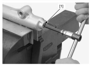
Remove the dust seal [1] from the fork slider.
