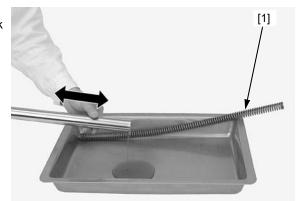
Hold the fork slider in a vise with a piece of wood or soft jaws to avoid damage.
