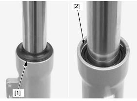
Check that the fork pipe moves smoothly in the fork slider. If not, check the fork pipe for bending or damage, and bushings for wear or damage.
