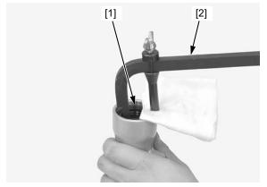
Remove the back-up ring [1] from the fork slider.
