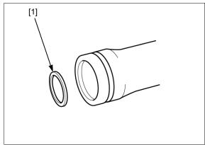
Remove the fork piston [1] and rebound spring [2] from the fork pipe [3].
