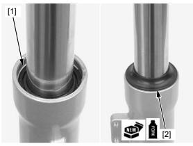
Pour half of the required amount of the recommended fork fluid into the fork pipe.
