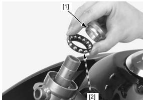
Remove the steering stem [1] from the steering head pipe.
