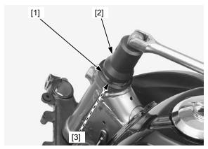
Remove the upper bearing inner race [1] and upper bearing [2].
