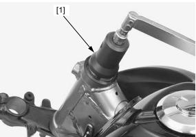
Install the top bridge [1]. Temporarily install the front fork (page 14-20). Install the steering stem nut [2] and washer [3]. Tighten the steering stem nut to the specified torque with a special tool.
