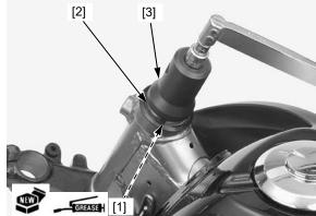
Turn the steering stem right and left to the end at least five times to seat the bearings.
