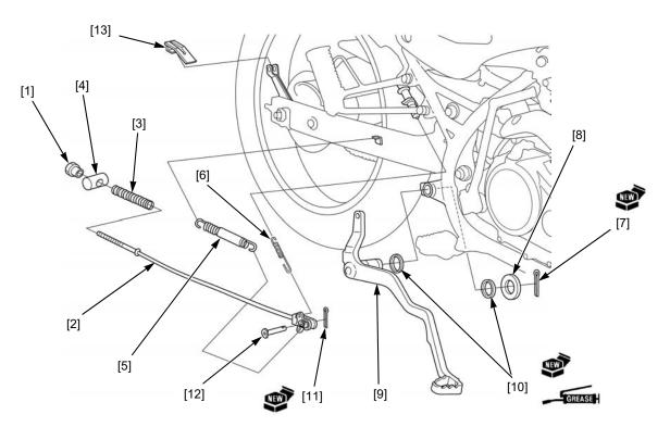
Apply grease to new dust seal lips.
