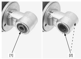
Press the needle bearing [1] out using the special tools and a hydraulic press.
