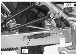
Remove the drive chain adjusters [1].
