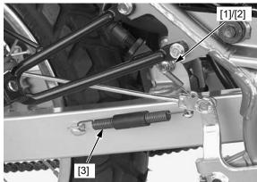
Install the carburetor drain hose [1] and crankcase breather hose [2] through the guide [3]. Install the drain plug [4] to the breather drain hose.
