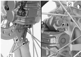
Install the pad pin [1] by pushing the pads against the pad spring to align the pad pin holes in the pads and caliper.
