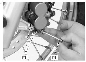
Make sure the pad spring is installed in position.
