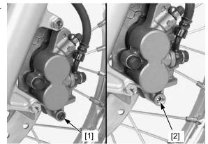
Remove the pad pin [1] while holding the brake pads [2], then remove the brake pads.
