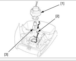
Remove the position light bulb socket [1]. Push the position light bulb [2] in, turn it counterclockwise and remove it.
