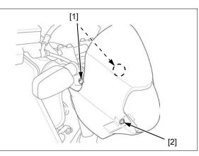
Remove the dust cover [1]. Unhook the bulb retainer [2]. Push the headlight bulb [3] in, turn it counterclockwise and remove it.
