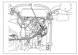
Disconnect the speedometer cable [1]. Remove the nuts [2], washers [3] and combination meter assembly [4].
