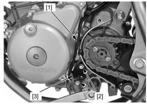
Remove the pin [1] and spring [2] from the shift drum. Installation is in the reverse order of removal.
