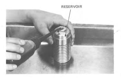
Install the O-rings on the hose joints. Fill the hose with ATF.
