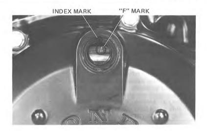
The index mark should be between the advance marks at 3,500 rpm.
