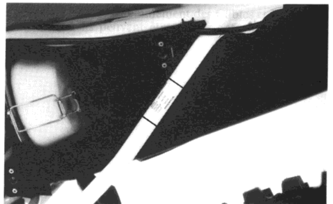
The color code label is attached to the left frame tube under the seat. When ordering a color coded part, always specify its designated color code.
