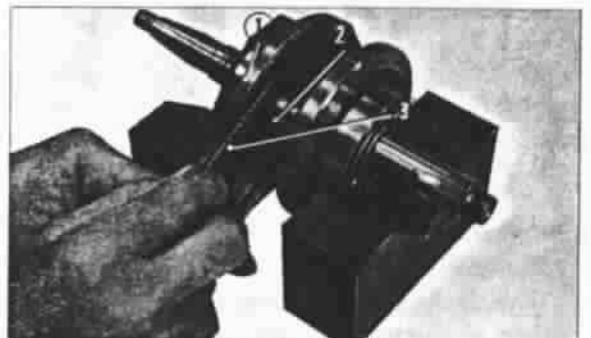
① Crankshaft ② Connecting rod ③ Thickness gauge Fig. 41
